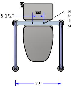
Mounts to toilet seat mounting holes. Toilet seat mounts on top of cross bar.
